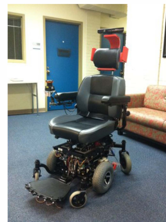
Figure 1: Wheelchair equipped with sensors modules has the framework necessary for semi-autonomous navigation
