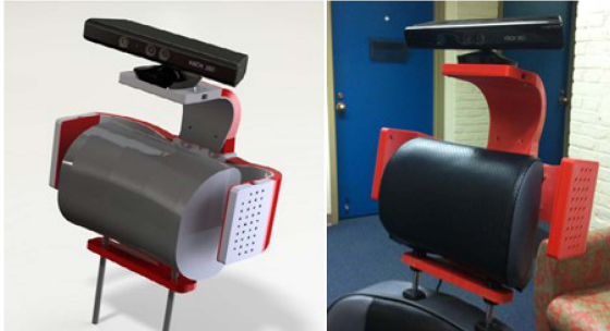
Figure 5: Configurable sensor and hardware mount on headrest, rendering (left) and finished product (right)
