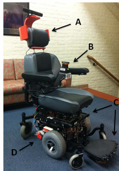
Figure 9: (A) Headrest sensor & hardware mount, (B) Configurable LiDAR module (not discussed within this paper), (C) IR and Ultrasonic sensors interfaced through sensor module, (D) Wheel-on-wheel encoder module
