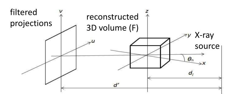
**Weighted Projection**: Weighted and ramp filtered raw data produce filtered projections  $Q_1, Q_2, ..., Q_K$ , collected at an angle  $\vartheta_n$  where  $1 \le n \le K$ .  $d_i$  = distance between the volume origin and the source. F(x, y, z) = value of voxel (x, y, z) in volume F. Volume F in xyz space and Projections are in uv space.
