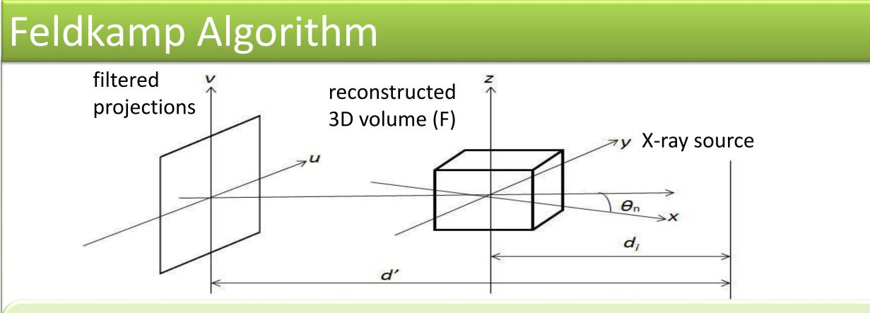
Weighted Projection: Weighted and ramp filtered raw data produce filtered projections  $Q_1, Q_2, ..., Q_K$ , collected at an angle  $\vartheta n$  where  $1 \le n \le 1$ K.  $d_i$  = distance between the volume origin and the source. F(x, y, z) = value of voxel (x, y, z) in volume F. Volume F in xyz space and Projections are in *uv* space.
