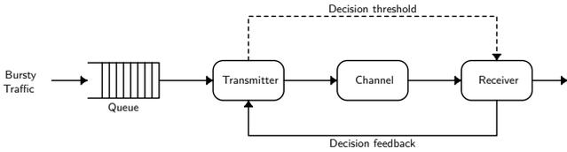
Fig. 1: Model of a transmitter with decision feedback
