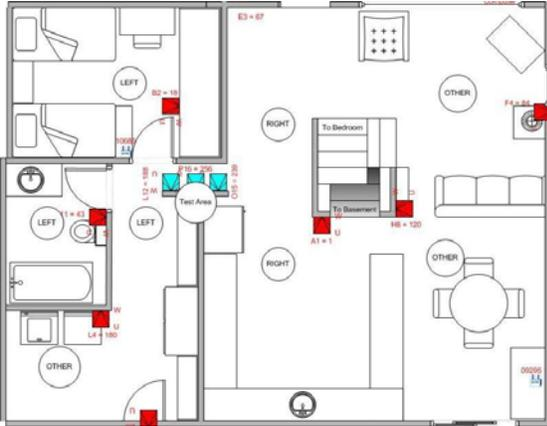
Fig. 1. Example of a part of a residence with a number of PIR sensors, RFID receiver stations and the test area.
