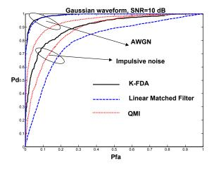
Figure 3: ROC curves for K-FDA, MF and QMI. Gaussian pulse, AWGN, SNR=5 dB.
