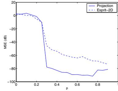
**Fig. 6.** MSE of the estimated angles  $\hat{\theta}_{ij}$ ,  $j = 1, \dots, 4$  as a function of the sparsity factor ( $p$ ) of the sources using both Esprit-2D (solid-line) and  $m - 1$  projections (dashed-line) for an scenario with two sensors and four sources.
