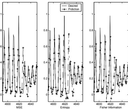
Figure 2. A sample collapse point in the test set from the laser time-series. Actual and predicted values for MSE, MEE, and EFI trained TDNNs in open-loop testing.
