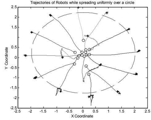
Fig. 2. Trajectories of robots while spreading themselves uniformly over a circle
