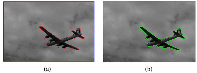
Fig. 5. Example of continuous edge map results. (Left) Result of the fixed-point iterations and (right) the final result are shown. (a) Result of the fixed-point algorithm for the BISB image. (b) Final result after interpolations along the ridge of the pdf (see in color).
