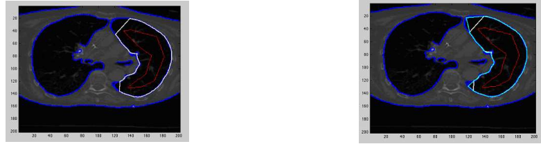
Figure 4.2: Two examples for the optimal interpolating curve with the edge probability density, where the big circles represent the points on the snake and interpolating curve combine these points
