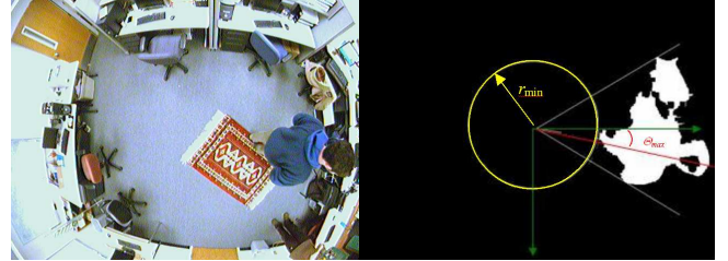
Figure 2. The view from fish-eye camera (left) and object localization from foreground segmentation (right). On the right, the segmented foreground object is assumed to be a standing person whose feet are centered at a small radius and an angle determined by the mode of the angular density of pixels in the cluster. The mode enables robustness to the inclusion of attached objects such as the chair that the person is moving in this frame.
