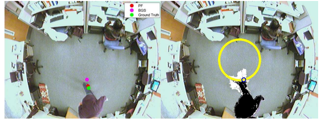
Figure 1. A typical output frame showing the results of foreground object detection based on the GMM background model with shadow removal (right) and estimated object location based on particle filter with background subtraction (BGS) result (left). On the right, black cluster is the moving object and white cluster is the estimated shadow.
